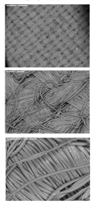
Fig. (1). Scanning electronic microscope pictures of a fabric impregnated with copper oxide particles. Yarn in weft contains the copper oxide particles (white dots).
